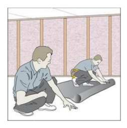
**Roll Out MLV** Roll out the MLV on the floor and mark the measurement from the previous step.
